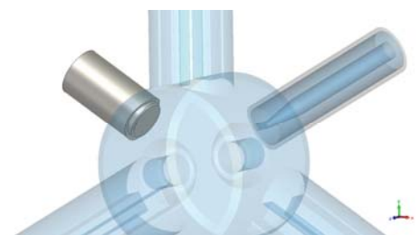
Fig. 1: Accelerating cavity with power coupler, tuner and higher order mode couplers
